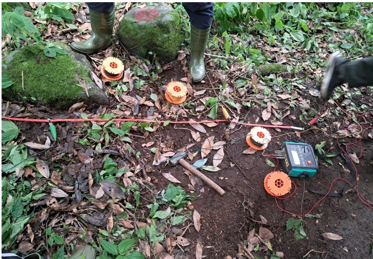
Figure 17: Soil resistivity test of Transmission line
