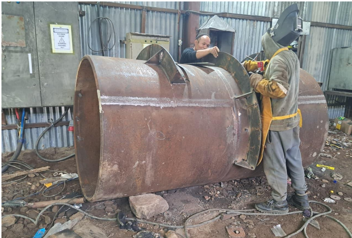
Figure 13: Preparation of AB 9 bend in HM workshop
